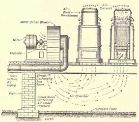
Fig. 247.—An air-blast-transformer installation.
